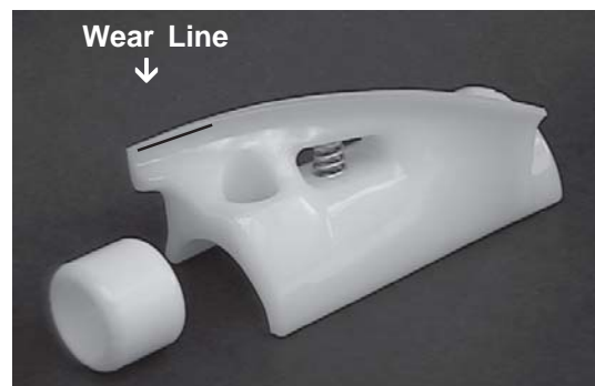
Figure 16. Auger Flight Wear & Front Auger Support Bushing Wear
