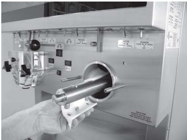
Figure 18. Auger Flight Removal
